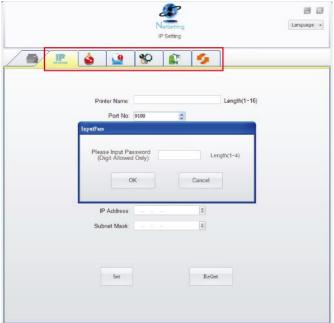
There are six tabs on the top of interface which can configure different types of network settings. But for the data security reason, you need correct password to enter the configuration pages.
