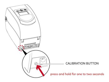
Press C-button for 2 seconds, it will make an auto-sensing to calibrate the label and ribbon's parameters.
