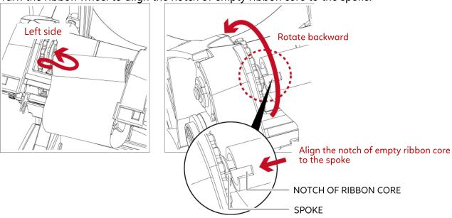
4. Turn the ribbon rewind wheel to tighten the ribbon until it has no wrinkles. The ribbon loading is completed once the ribbon supply module and ribbon rewind module are assembled correctly.
