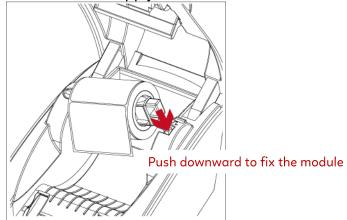
4. A new label supply module is completed.
