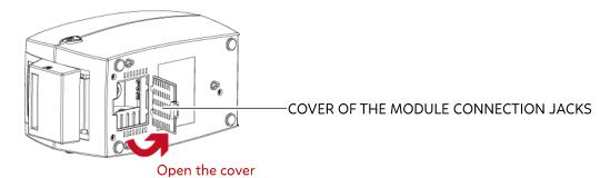
7. Plug the connector for the cutter to the jack.
