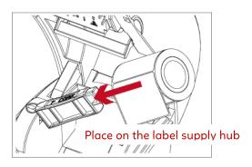
3. Push the label supply module downward and close the release catch.
