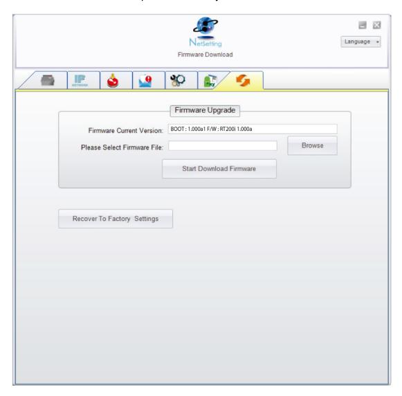
In addition to the firmware update, you can press "Recover To Factory Settings" button to restore the printer configurations back to factory default.
