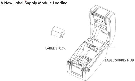
1. Unlock the release catch to lift the label supply hub.
