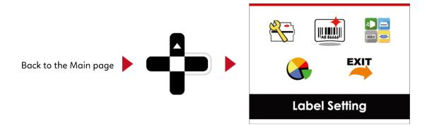
On MAIN PAGE, select the "EXIT" icon and press the FEED button to exit from SETTING MODE and the printer goes back to READY status.
