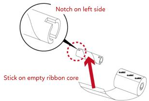
2. Wind the ribbon around the empty ribbon core for 2 to 3 circles.
